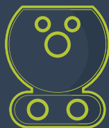
CCS 50kW DC
